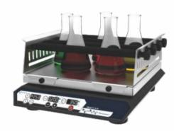
Max. 500 RPM, 10 mm Ø (PS10), Max. 300 RPM, 20 mm Ø (PS20)
